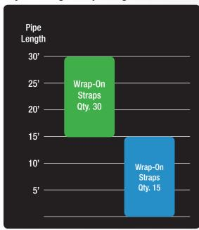
For additional pipe lengths, we recommend 1 strap per foot of pipe length.
